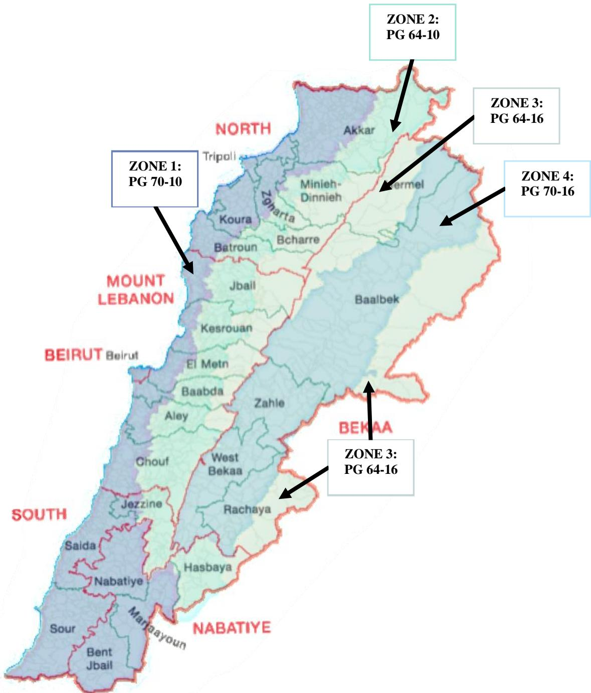
**B.3** A one-grade increase, equivalent to 6°C, shall be applied to the base high-temperature PG grade in cases of slow traffic (between 20 km/h and 70 km/h) or standing traffic (<20 km/h). Over and above, a one-grade increase shall be applied to the base high-temperature where traffic volume exceeds 10 million ESALs as specified in Table 4.1.3.
